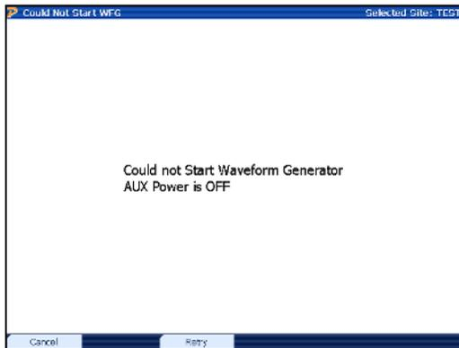
The PowerMaster® cannot detect an auxiliary power source between 100-530VAC. Check the connections and/or verify the Auxiliary Power switch is in the "on" position (- = on).
