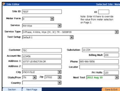
In Site Editor, tab to "Test Setup" then press F4
