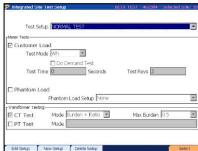
Select then press F2 to edit the Test Setup
