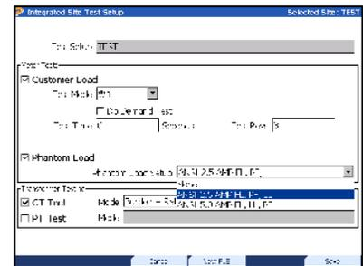
Tab to "Phantom Load Setup," select correct PLS, then press F5
