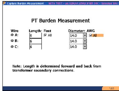
Input the total length and diameter (AWG). Press F6 to continue.
