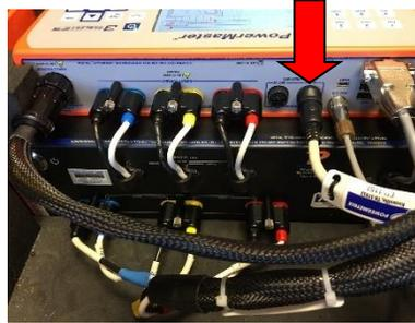
Connect Current Probe Adapter cable to PROBE SET 1. Connect probes to cable ends.
