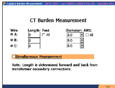
Verify Length is set to 0 and “Simultaneous Measurement” is NOT selected. Press F6 to continue.
