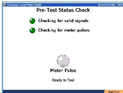
Wait for meter pulse, then press F6 "Start Test"
