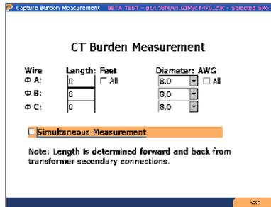
Input the total length and diameter (AWG). Verify "Simultaneous Measurement" is NOT selected. Press F6 to continue.
