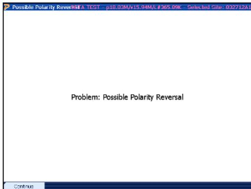
The PowerMaster® detects a phase angle error between 190 and 170 degrees for the phase under test. Attempt the following:
