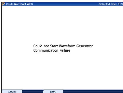
The PowerMaster® cannot communicate with the WFG board. Attempt to power off/on to fix the issue. If this is not successful, contact Technical Support.
