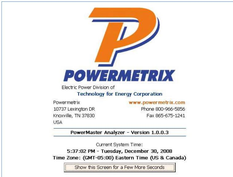
At power up, the PowerMaster® displays a “splash” screen briefly. If the user has a USB mouse connected to one of the USB Peripherals, the screen can be paused for 10 more seconds. After the 10 seconds are complete, the analyzer will boot up to the main menu as normal.
