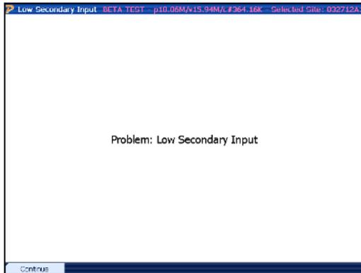
The PowerMaster® detect less than 0.1A secondary current on the probe used for the phase under test. Check the following:
