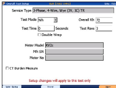
On PowerMaster, enter Kh and test parameters. Press F6 to continue.
