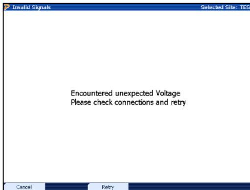
The PowerMaster® sees a voltage signal that is  $\pm 0.5\%$  beyond the desired amplitude. Verify the following:
