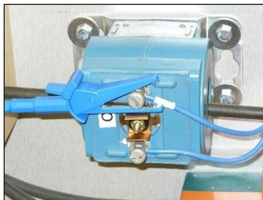
Connect the blue (+) voltage cable connection to the CT secondary for C phase
