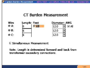
Input the total length and diameter (AWG). Verify "Simultaneous Measurement" is selected. Press F6 to continue.
