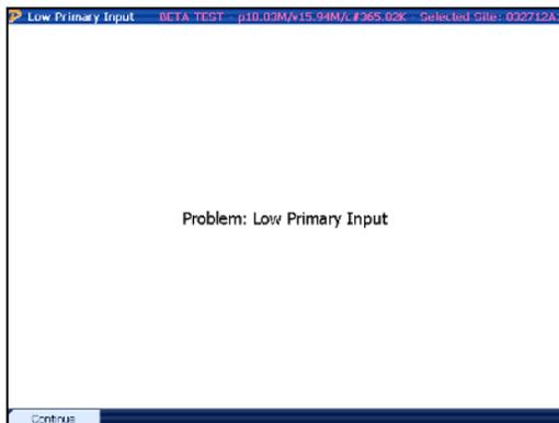
The PowerMaster® detect less than 0.1A primary current on the probe used for the phase under test. Check the following:
