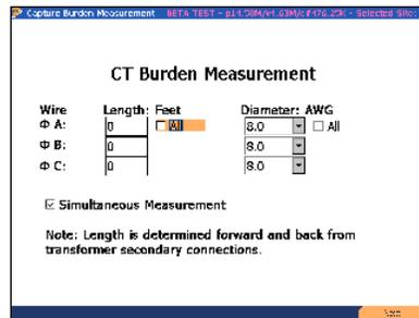
Verify Length is set to 0 and "Simultaneous Measurement" is selected. Press F6 to continue.
