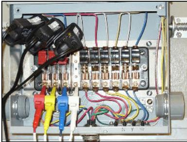
Clamp current probes around voltage wires at test switch. Connect voltage leads as normal.
