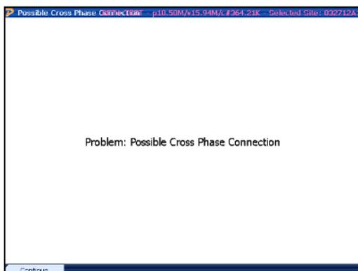
The PowerMaster® detects a phase angle error greater than 100 degrees for the phase under test. Attempt the following:
