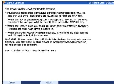
Insert USB Flash drive into a USB peripheral and press F3 to scan. Verify unit is plugged into AC Power.
