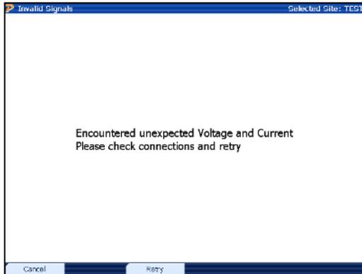
The PowerMaster® sees a voltage signal AND a current signal. Check the connections.
