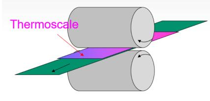
Measurement of heat distribution between lamination rollers
