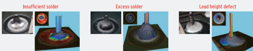
Flow solder/insertion component inspection examples
