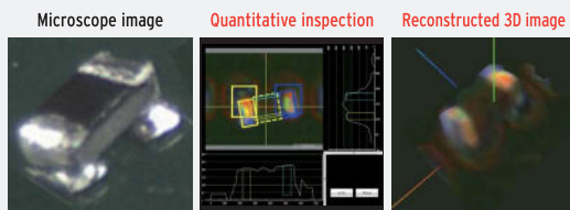
Micro component (0402) offset defect
