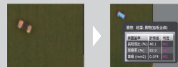
Foreign object (0402 scattered chip) detection example
