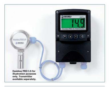
The Intrinsically Safe Field Display is a 4-digit loop-powered local monitor for the Easidew PRO I.S. and Easidew I.S. transmitters. It is certified with ATEX, IECEx, UKCA, and FM and housed in an IP66 enclosure with a terminal compartment for wiring. The measurement unit can be labelled as ppm, ppm<sub>w</sub>, °C dp or °F dp.
