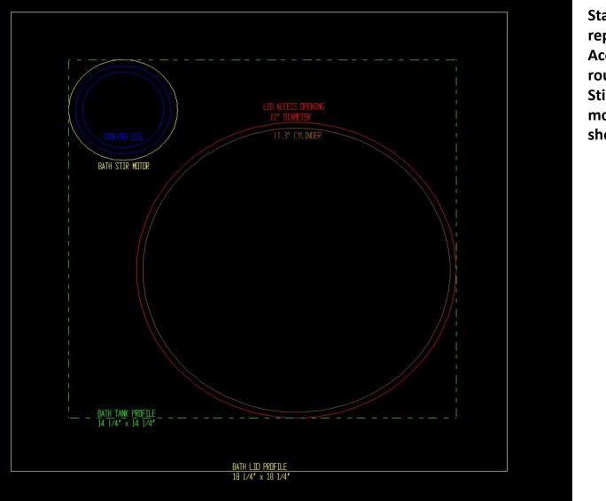
Standard bath lid will be replaced by this design. Access opening will be round (12" in diameter). Stir motor will be mounted in the corner as shown.
