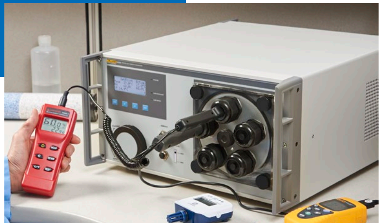
Figure 1. Typical 5128A RHapid-Cal setup for calibrating humidity sensors
