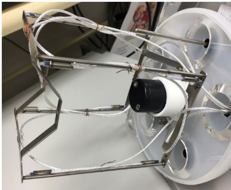
Figure 5. Calibration jig placed in the 5128A during factory calibration. Seven sensor test points at twelve different combinations of humidity and temperature set points are tested in the chamber to ensure 5128A performance.
