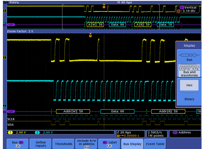
I 2 C bus setup, showing selection of bus display modes.
