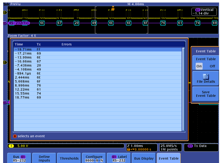
Event table for RS-232 bus with all captured packets time stamped and in a tabular view.
