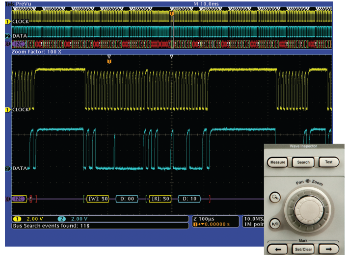
Search – I2C decode showing results from a Wave Inspector® search for Address value 50. Wave Inspector® controls provide unprecedented efficiency in viewing and navigating waveform data.
